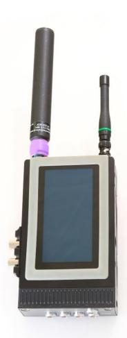
The transmitter comes equipped with a built-in camera control module which makes the unit capable of wireless Camera Control Unit (CCU) functionality when paired with the Real Freedom Receiver's optional UHF data module. With the CCU functionality built into the transmitter, the unit is more streamlined and easier to deploy.
