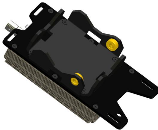
Figure 4: Data transmitter ¼-20 UNC mounting screws (yellow)
